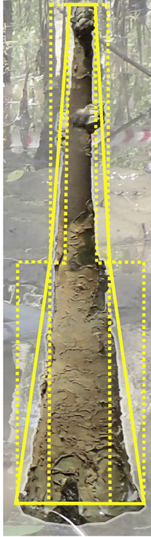
Fig. 4. Illustration of the error bounds for manual measurements. Diameters were measured at three locations: basal, middle and top. These measurements were linearly interpolated to estimate stem diameters at all elevations (solid lines). Upper and lower bounds on diameter were obtained by neglecting taper between measurement elevations (dotted vertical lines). In this particular example, the true diameter lies in between the “linear” and the “min” estimates, but in some other cases (not shown) the true diameter was between “linear” and “max” estimates.
