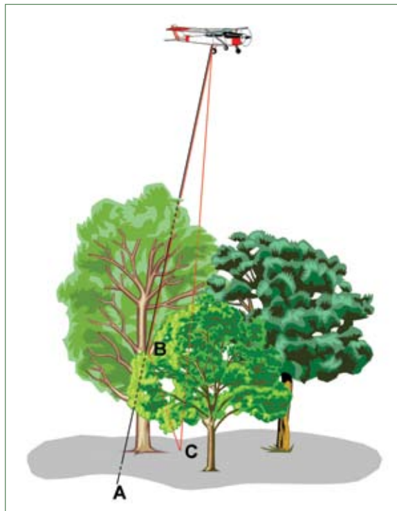
Figure 7—Illustration of LIDAR path reflectance. Black line represents the beam propagation anticipated by the LIDAR instrument. Red line represents the actual beam propagation. Letters A, B, and C indicate the locus of anticipated return, first, and second beam inflection points, respectively.
